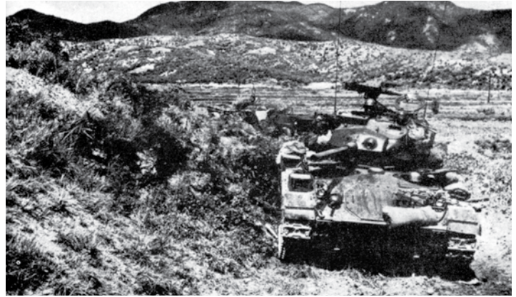
Developed as a light tank in WWII, the M24 was the only tank available to American forces when the North Koreans launched their invasion. It was no match for the T-34/85.
